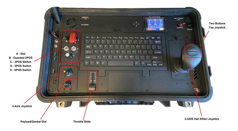
The control/transmitter interface is highlighted above. The GCS SmartView™ interface allows the end-user to assign channels and functions to the various highlighted hardware. If necessary there are trim buttons to the left of the flight control stick. Note the throttle trim above the throttle slide.
