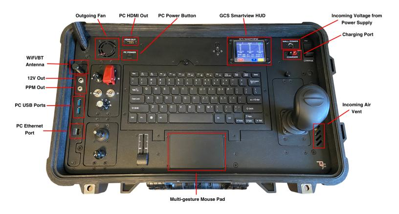
The MIRA 12X was designed to work with your existing ground components and future UAV technology. Everything is strategically laid out for easy/quick access. As with any new component it is best to rigorously test before performing critical flights/missions.
