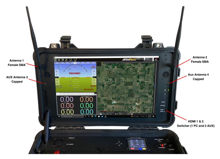
NOTE # 1 - DISPLAY STARTUP: The MIRA 12X HDW version's embedded PC auto-turns on when MASTER power is switched to 'ON'. It may take 3 to 5 seconds for the 19" display turns on and shows Window Startup prompts. ALWAYS press PC POWER when turning off GCS so embedded PC turns off appropriately.
