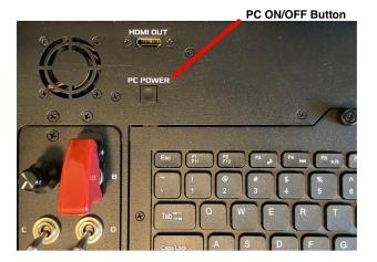
The MIRA 12X has an integrated OnLogic<sup>™</sup> HX500 Embedded PC with Intel<sup>™</sup> microprocessor. The MIRA 12X has an integrated power switch on the switch panel. When turning the MIRA 12X on, the PC system does not turn ON until you press the PC POWER for the Dual Screen HD version. For the Single Screen HDW version the PC will automatically turn on when MASTER Power is pressed to ON position.
