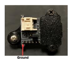
PPM/S-Bus and +5V IN from 12PCX 3POS JST XA Connector
